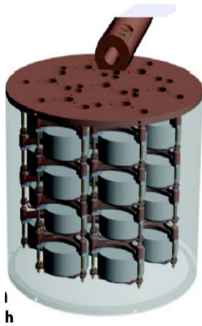
Multiple Ge arrays in a single dewar
