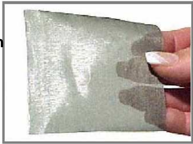
Figure 1: Micronic Mesh: 1 mil wires with 400 wires/inch
